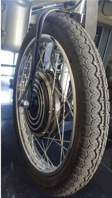
Figura 6.2: Motor BLDC In-Wheel Rueda DD
