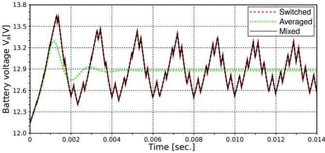
Fig. 13. Battery voltage trajectory (startup).
