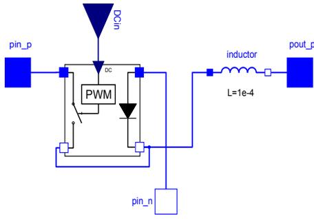
Fig. 7. Modelica mixed model of a Buck converter.
