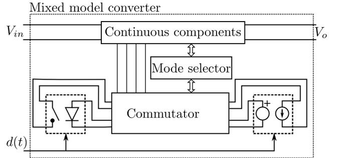
Fig. 4. Mixed model schema of a DC/DC converter.
