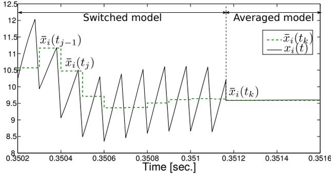
Fig. 5. Detail of the current in the Buck converter when the hybrid model switches from the switched to the averaged submodel
