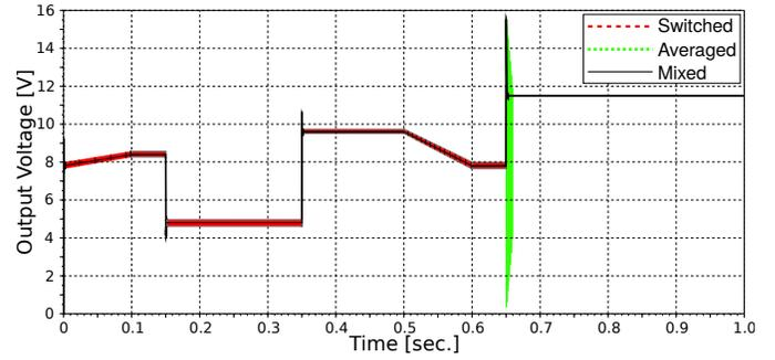
Fig. 9. Buck converter output voltage.
