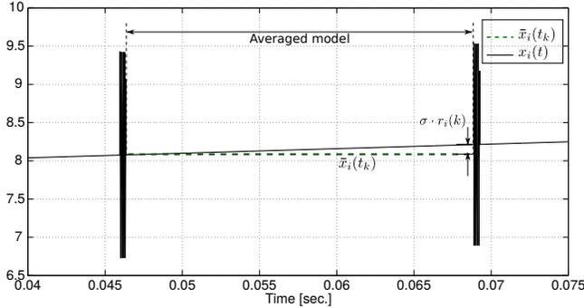
Fig. 6. Detail of the current in the Buck converter when the hybrid model switches from the averaged to the switched submodel
