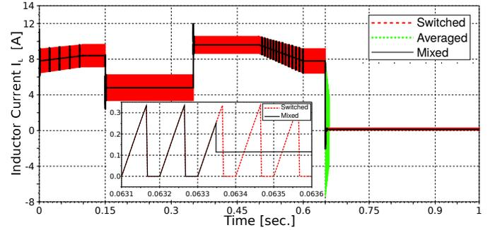
Fig. 10. Buck converter inductor current.
