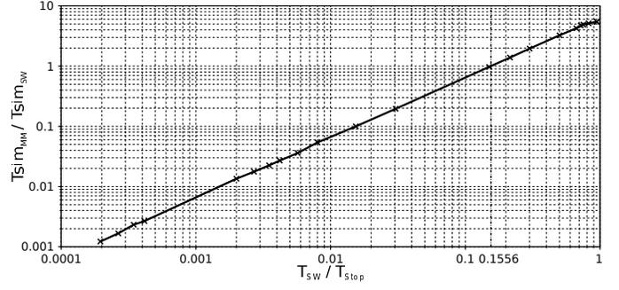
Fig. 11. CPU time of mixed mode and switched models vs. fraction of time in transient operation.
