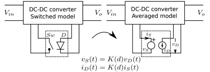
Fig. 2. Averaged model approximation of a DC-DC converter.
