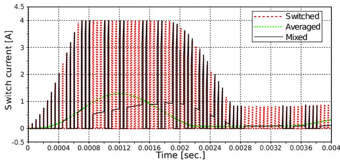
Fig. 16. Switch Current Startup in the Regulated Buck Model
