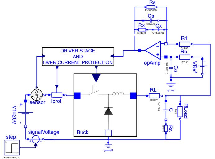
Fig. 14. Modelica model of a regulated Buck.
