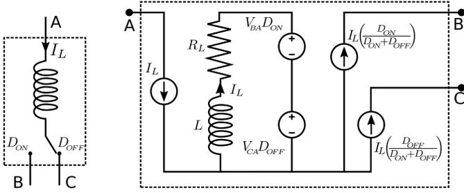
Fig. 3. Switched Inductor: a) Real configuration b) Unified switched inductor averaged model
