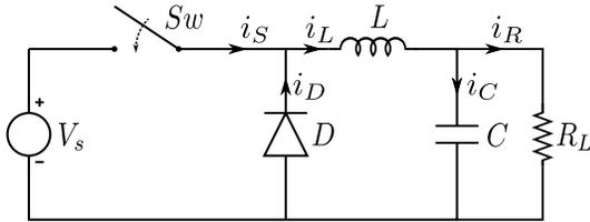
Fig. 1. Buck converter circuit
