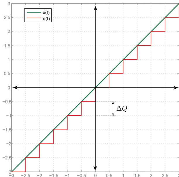
Figure 1: Quantization function  $q(x)$  with quantum  $\Delta Q = 0.5$
