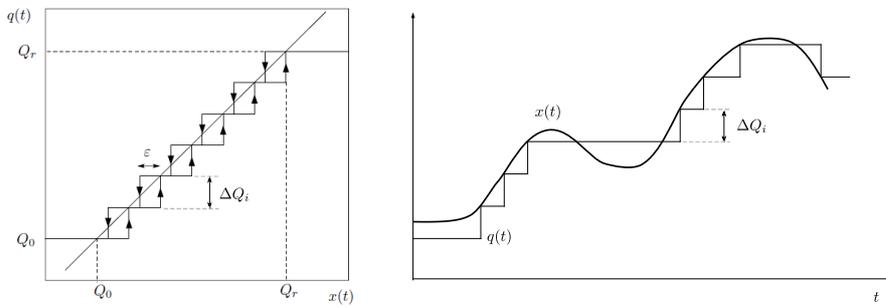
Figure 3: Quantization function with hysteresis (left) and hysteretic quantization with hysteresis width  $\varepsilon = \Delta Q$  (right)
