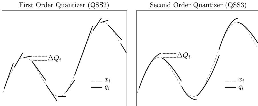
Figure 5: First order quantization function (QSS2, left) and second order quantization function (QSS3, right)
