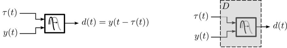
Figure 7: Delay block (left). Delay DEVS model  $D$  (right)
