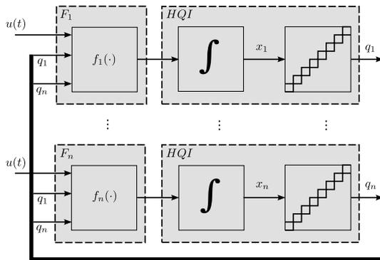
Figure 4: Block diagram representation of a QSS. Arrow references: thin (single component signal), bold (multiple component bus).
