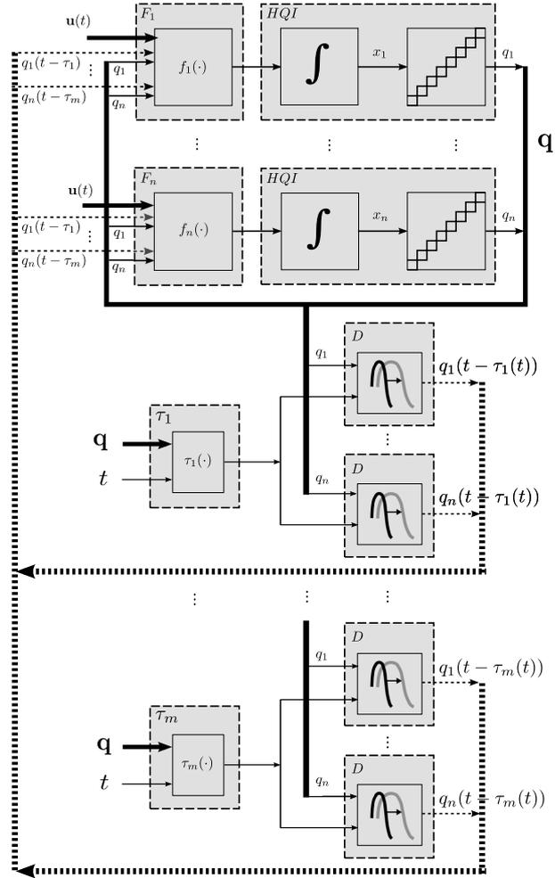
Figure 6: Block diagram representation of a DQSS. Box references: continuous (regular block), dotted (DEVS equivalent model). Arrow references: thin (single component signal), bold (multiple component bus), continuous (non-delayed), dotted (delayed)
