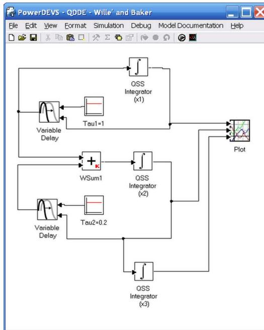
Figure 10: Model of a DDE implemented in the PowerDEVS tool
