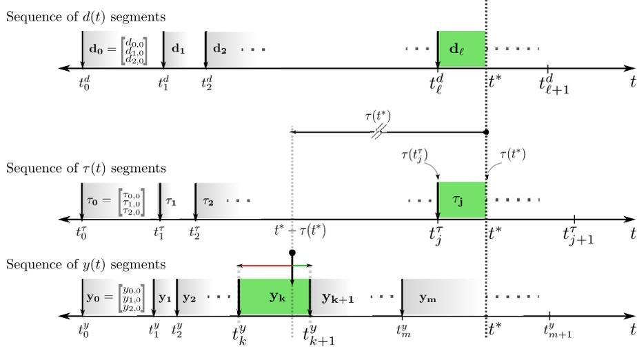
Figure 8: DQSS algorithm based on polynomial segments. Sequences of time instants and polynomial coefficients.
