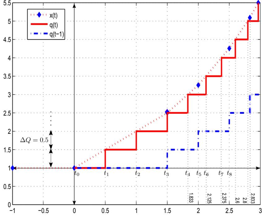
Figure 2: Solution of  $x(t)$  for a DDE approximated by Eq. (4)
