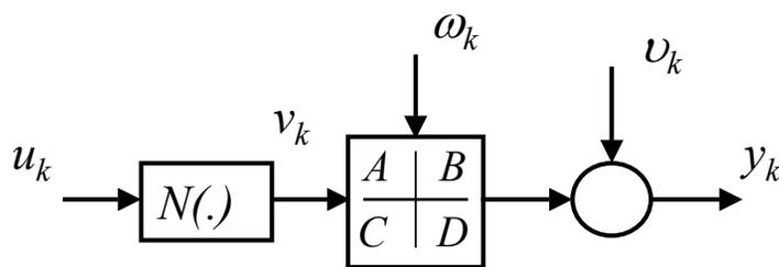
Fig. 5: Hammerstein model
