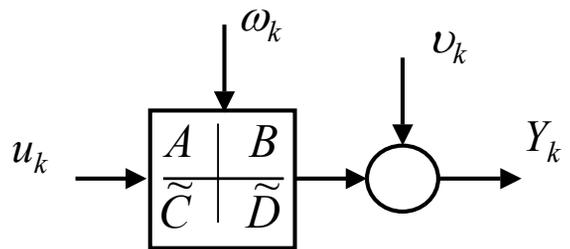
Fig. 8: Equivalent LTI model with output  $Y_k$
