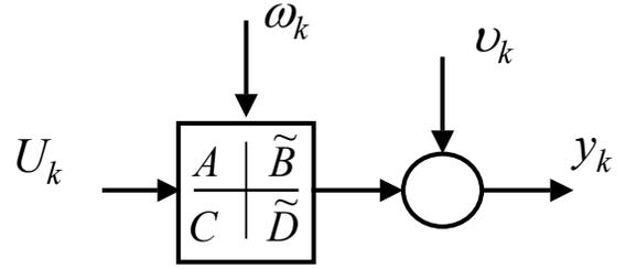
Fig. 6: Equivalent LTI system with input  $U_k$
