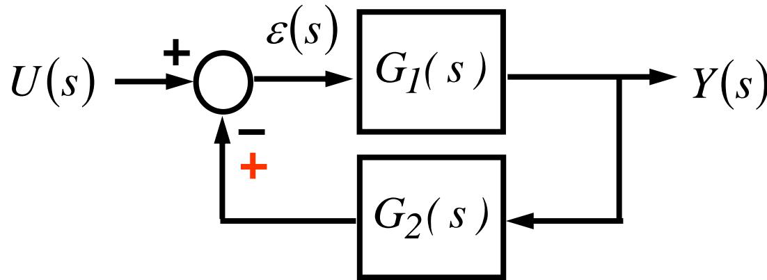
$$\begin{cases} \varepsilon(s) = U(s) - G_2(s)Y(s) \\ Y(s) = G_1(s)\varepsilon(s) \end{cases} \rightarrow \begin{aligned} Y(s) &= G_1(s)[U(s) - G_2(s)Y(s)] \\ &= G_1(s)U(s) - G_1(s)G_2(s)Y(s) \\ Y(s)[1 \pm G_1(s)G_2(s)] &= G_1(s)U(s) \end{aligned}$$
