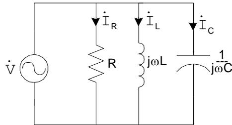
$$\begin{aligned} R \quad \tilde{S}_R = P_R = \frac{V^2}{R} \quad Q_R = 0 \\ L \quad \tilde{S}_L = jQ_L = j \frac{V^2}{\omega L} \quad P_L = 0 \\ C \quad \tilde{S}_C = jQ_C = j \omega C V^2 \quad P_C = 0 \end{aligned}$$
