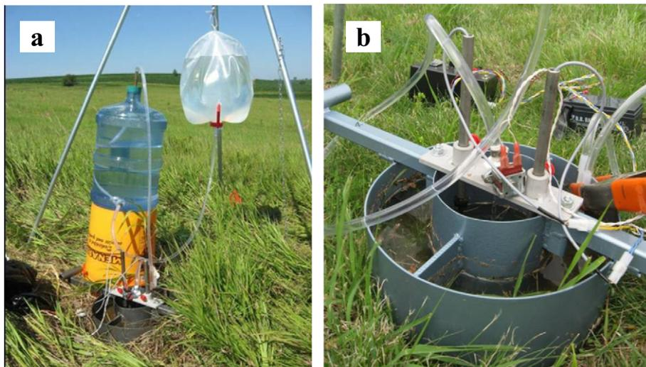
Fig. 2. The semi-automated double ring infiltrometers: (a) A complete view of the DRI system; (b) a close-up view of the infiltrometer.
