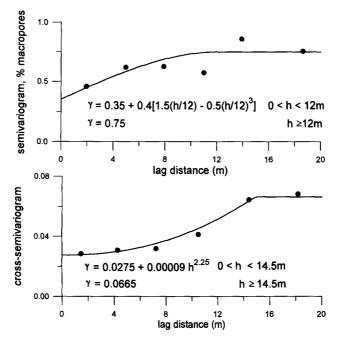
Fig. 7. Experimental and fitted theoretical semivariogram of ln-transformed depth-averaged blue stained area (in % of total area) (top), and cross-semivariogram between  $\ln(K_s)$  and ln-transformed depth-averaged blue stained area (in % of total area) (bottom). Type-II columns were used for this purpose.
