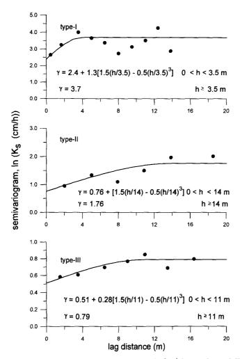
Fig. 6. Experimental and fitted theoretical semivariogram of  $ln(K_S)$  for sample type I, II, and III.
