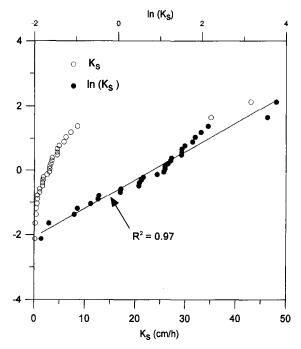
Fig. 2. Fractile diagram of  $K_{\rm S}$  measured on type-II cores for raw and In-transformed data.
