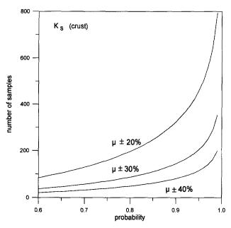
Fig. 3. Number of samples necessary to estimate the mean within 20, 30, or 40% of the true mean of  $K_s$ , for different probability levels.
