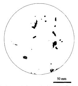
Fig. 4. Example of a digitized photograph of cross-sectional view of a soil column showing cylindrical and elongated macropores.
