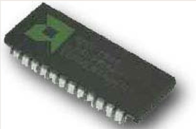
DIP (Dual In-line Package) Device
