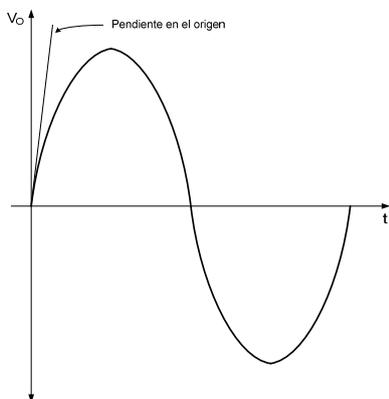
$$V_0(t) = V_{0M} \text{ sen}(2\pi f t)$$
