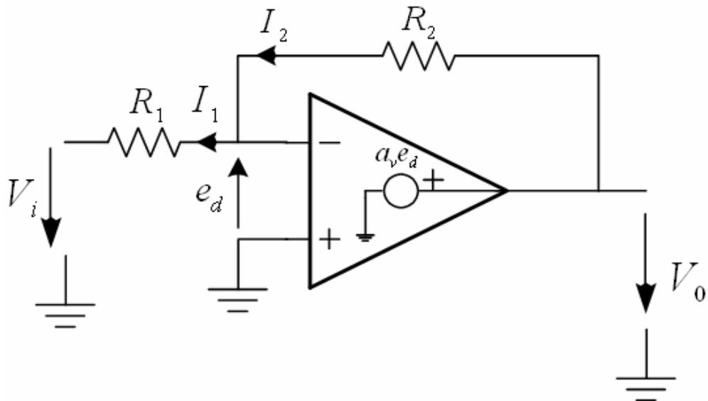
$$\left. \begin{aligned} V_0 &= a_v e_d \\ e_d &= -e^{(-)} \\ e^{(-)} &= \frac{R_2}{R_1 + R_2} V_i + \frac{R_1}{R_1 + R_2} V_0 \end{aligned} \right\} V_0 = -a_v \frac{R_2 V_i + R_1 V_0}{R_1 + R_2}$$
