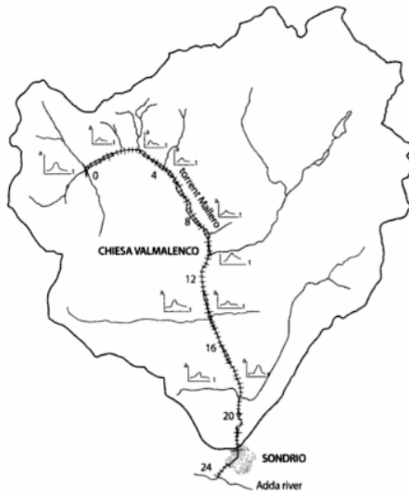
Figure 2: Basin of the torrent Mallero and model schematization.
