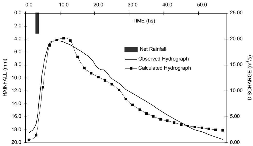
Fig. 14. Observed and calculated hydrographs for Ludueña river basin. Event without overflow
