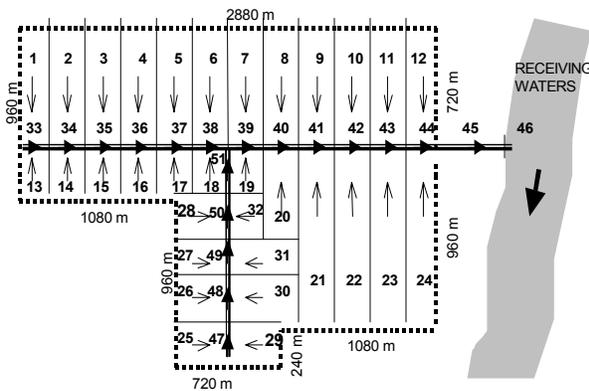
Fig. 3. Topological discretization of surface layer
