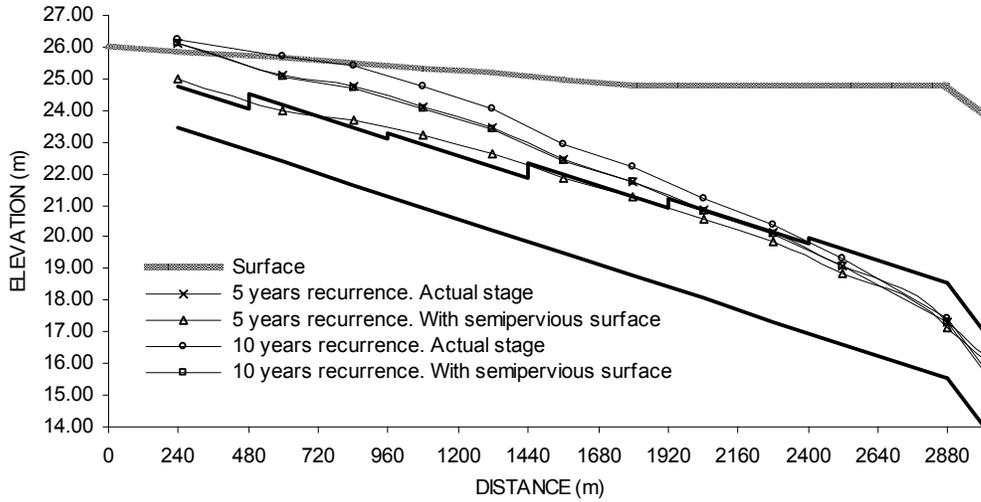
Fig. 6. Calculated water levels in trunk conduit
