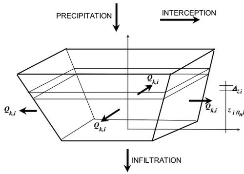
Fig. 1. Continuity equation of a cell
