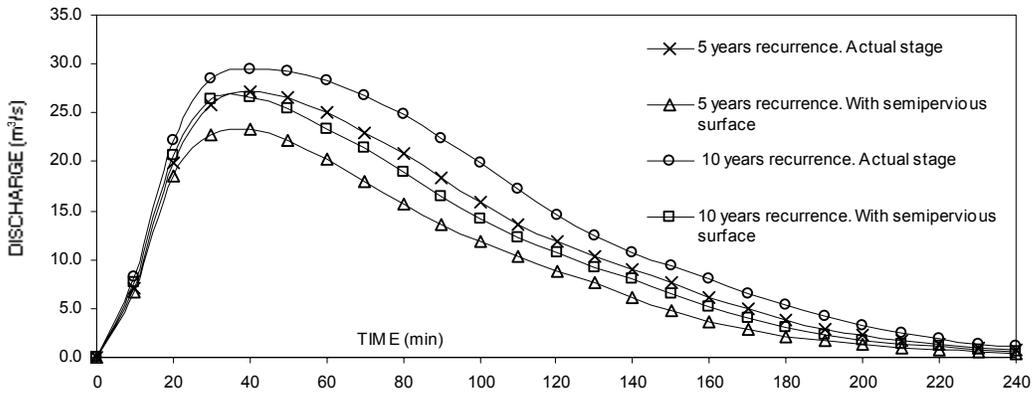
Fig. 5. Calculated net hyetographs and hydrographs. Actual and with semipervious surface stages
