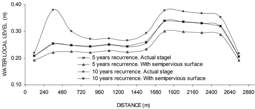
Fig. 7. Calculated water levels over the main avenue
