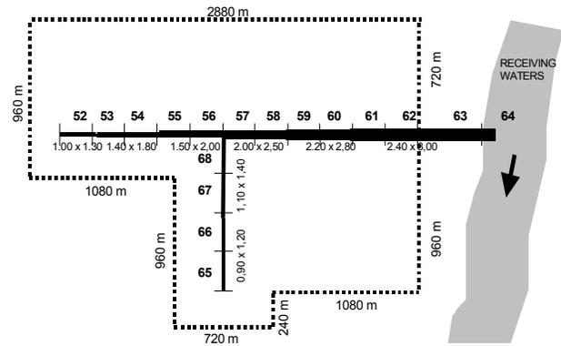
Fig. 4. Primary network of close conduits
