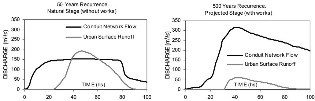
Fig. 10. Downstream hydrograph. 50 and 500 years recurrence
