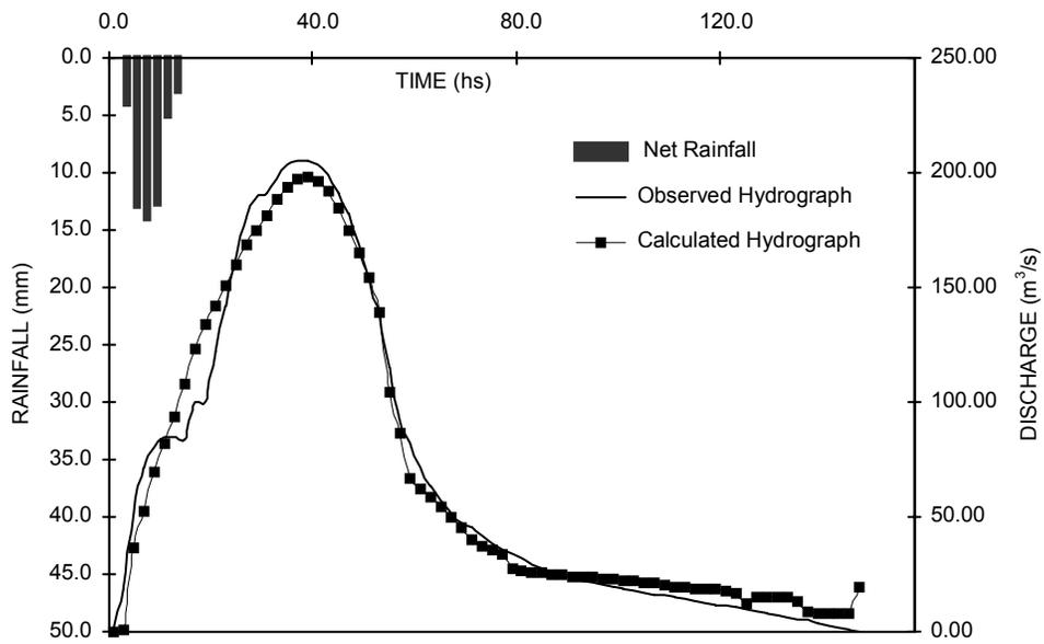
Fig. 15. Observed and calculated hydrograph for Ludueña river basin. Event with overflow
