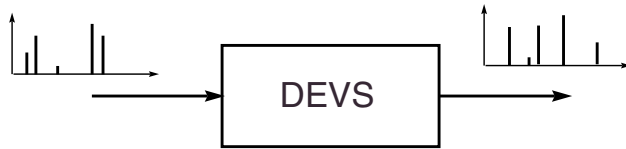
Figure 1: Input/Output behavior of a DEVS model
