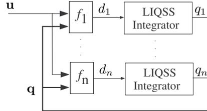
Figure 4: Block Diagram of LIQSS
