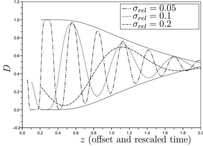
Figure 4: Envelope of the power peaks. The dotted and dashed lines represent the normalised power demand  $D$  for different values of  $\sigma_{rel}$  according to (9), all of them adjusted to the offset and rescaled time variable  $z$ . The continuous line is the envelope given by (11)-(12).
