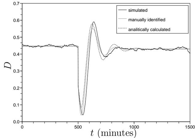
Figure 5: Step power response  $D$  for 10000 simulated ACs with parameters described in Table 1 ( $\sigma_{rel} = 0.2$ ) and using the second order systems calculated with (15) and identified manually.
