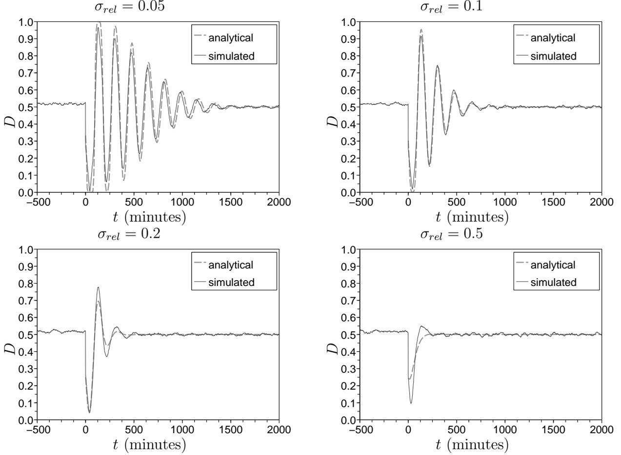
Figure 3: For different values of  $\sigma_{rel}$ , expected and simulated  $D$  (normalised power demand) response to an increase of  $0.5\text{ }^{\circ}C$  in all ACs' temperature set points. The simulated results are for 10000 ACs with log-normally distributed  $C$  and constant  $R$  and  $P$ , and were obtained using the parameters from Table 1. To obtain a duty cycle of 0.5,  $\theta_a$  was set to  $\theta_{ref} + RP/2 = 34\text{ }^{\circ}C$ .
