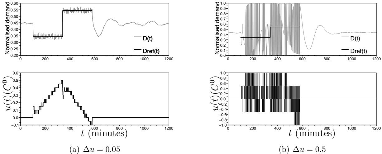
Figure 7: DSM scenario on a population of 10000 ACs between  $t = 100$  and  $t = 580$  (minutes). The control aims to make the normalised power output  $D(t)$  follow the reference signal  $D_{\text{ref}}(t)$  (top plot). The control signal  $u(t)$  is shown in the bottom plots. The quantisation of  $u(t)$  is  $\Delta u = 0.05$  for (a) and  $\Delta u = 0.5$  for (b).
