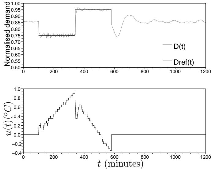
Figure 10: Normalised output power demand  $D$  (top) and global input control signal  $u(t)$  (bottom) for a DSM scenario between  $t = 100$  and  $t = 580$  (minutes) on a population of 10000 ACs with 85% mean duty cycle. The control aims to make the normalised power output  $D(t)$  follow the reference signal  $D_{ref}(t)$ . The 10000 ACs are divided into 10 clusters of 1000 ACs each. The bottom plot shows the global control signal.
