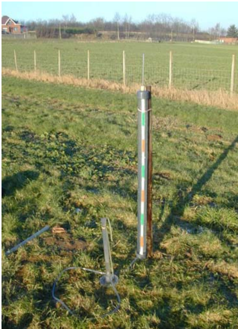
Figure 3.1 Single ring pressure infiltrometer set-up
