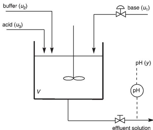
Fig. 1 Schematic representation of the pH neutralisation process
