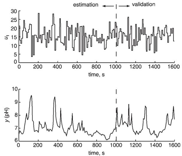
Fig. 5 Estimation (first 1000 points) and validation (remaining 600 points) input-output data
