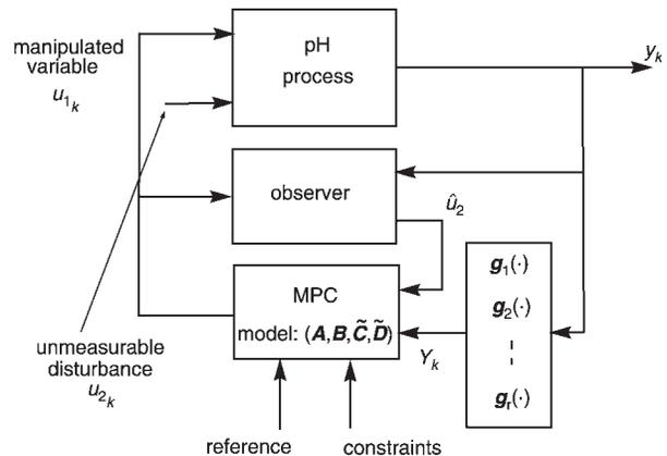
Fig. 9 [WMPC + observer] combined scheme
