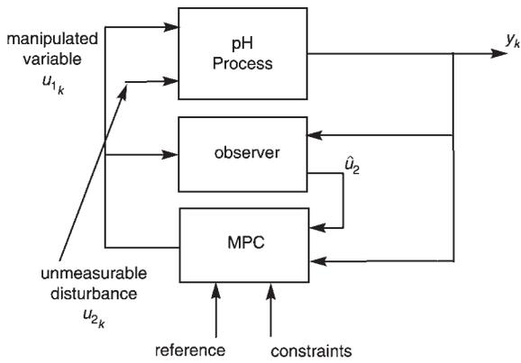
**Fig. 10** [Linear MPC + observer] combined scheme
