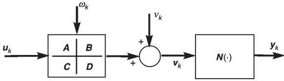
Fig. 2 Multivariable Wiener model
