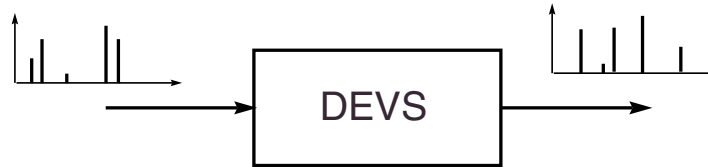
Figure 2.4: Input/Output behavior of a DEVS model
